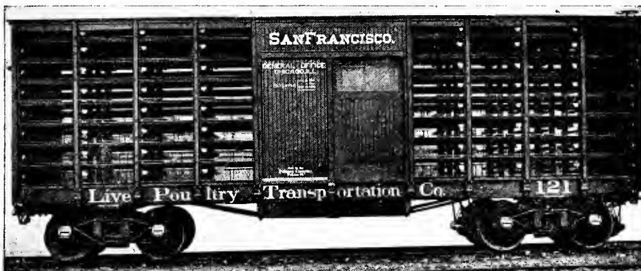
Fig. 8. POULTRY CAR. Length, 33 ft. 10 ins. Capacity, 16,000 lbs., 5,000 Fowl, 2,000 Geese, or 1,400 Turkeys. Equipped with Swing Motion Diamond Trucks.
